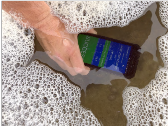
Figure 10. Servicing an EnvLogger underwater, with a waterproof (IP68) smartphone.
